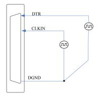
Figure 4.5 clock input and trigger Signal Connection
