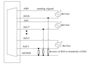
Figure 4.2 double-ended input connection
