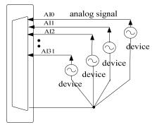
Figure 4.1 single-ended input connection
