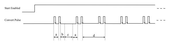
Figure 6.1 Grouping Sampling which grouping cycle No is 1 under the Internal Clock Mode
