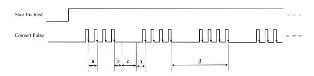
Figure 6.2 Grouping Sampling which grouping cycle No is 2 under the Internal Clock Mode
