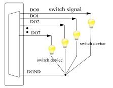
Figure 4.4 digital signal output connection
