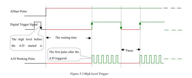
When ADPara.TriggerDir = USB2085\_TRIGDIR\_POSITIVE, it means the trigger level is high. When DTR trigger signal is in high level, A/D is in the conversion process, once the trigger signal is in the low level, A/D conversion will automatically stop, when the trigger signal is in the high level again, A/D will re-access to the conversion process, which is, only converting the data when the trigger signal is in the high level.
